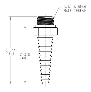
DIMENSIONS ARE IN INCHES AND [MILLIMETERS].
